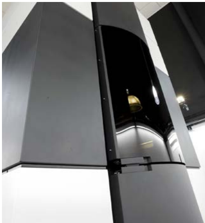
The PICO electron microscope can measure atomic distances and displacements to within one picometre.
