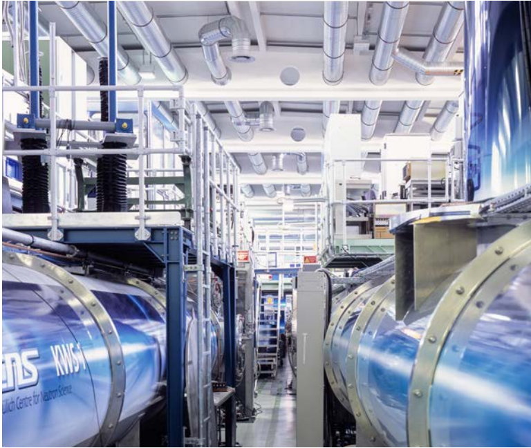
Small angle scattering instrument KWS-1 of Forschungszentrum Jülich at Heinz Maier-Leibnitz Zentrum in Garching (at the left)
